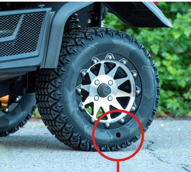
OTR'S innovative, patent-pending NDX tire lasts up to 2x longer than airless options, even when carrying extreme loads with a 1" hole in its sidewall.
